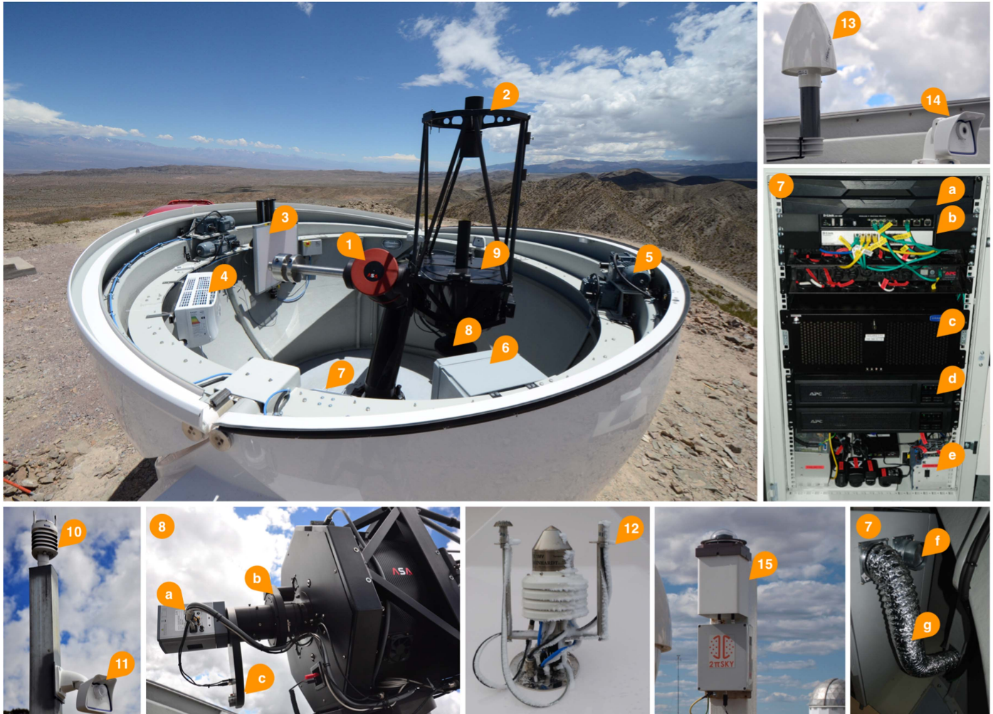
Figure 5. Solaris hardware overview. (1) ASA DDM160 telescope mount. (2) 0.5-m optical tube assembly. (3) Flat field screen and FlatMount lifting manipulator. (4) Air-conditioner internal unit. (5) Dome segment motors. (6) PLC HVAC and supervision system. (7) 19-inch rack cabinet: (a) KVM remote console with keyboard and LCD monitor; (b) network router and switch; (c) control PC; (d) UPS units, and (e) power supplies and accessories. (8) Imaging train: (a) Andor iKon-L CCD camera, (b) ASA field rotator, and (c) FLI filter wheel. (9) Mirror covers. (10) Vaisala WXT-520 weather station. (11) Mobotix external surveillance camera. (12) Reinhardt weather station. (13) Meinberg GPS antenna. (14) Mobotix internal surveillance camera. (15) SBIG all-sky camera with custom 2\pi Sky™ cloud detection module. Graphic based on original from Kozłowski et al. (2014). (A color version of this figure is available in the online journal.)
